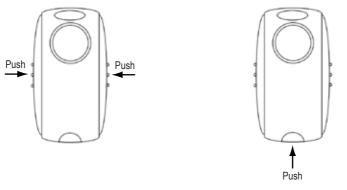
To sound the alarm press <u>both</u> sides simultaneously
